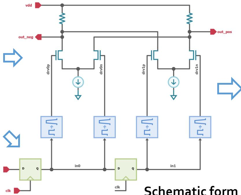
Timing accuracy of digital pulses is not limited by timestep
